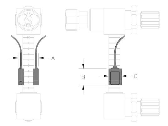
\*Electronic Sentinel may be mounted with wire up (as shown) or wire down (not shown).
